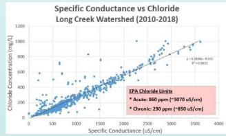
Figure 4: Conductivity and chloride correlation in the conductivity readings for the Long Creek Watershed South Branch
