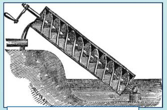
Hand Powered Archimedes Screw Pump.
