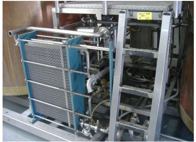
Make sure the heat exchangers are well maintained and regularly check the meter readings of the water flow. Pollution of the heat exchanger will negatively affect the heat transfer and cause an excess of water flow.
